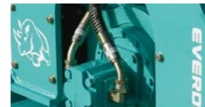
Oil bath type Compacted weight chamber is filled with gear oil. Therefore, old oil needs to be eliminated periodically. (Replacement interval is about 1 year)
